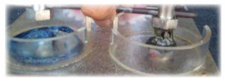
Left: After the impact test, the previously used grease (blue) splashes, showing it is not suitable for the load. Right: Pyroshield 5182 grease remains at the hammer head, which means a film layer remains to protect against the friction caused by metal-to-metal contact.
