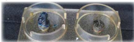
LE's Impact Tester (with 60-lb bar pressure) is used to check the grease's condition after applying an extreme load. Left: A sample of the previously used grease (blue) was taken from a new tube for testing purposes. Right: A sample of Pyroshield 5182 grease (brown) was taken from the twistlock after use.
